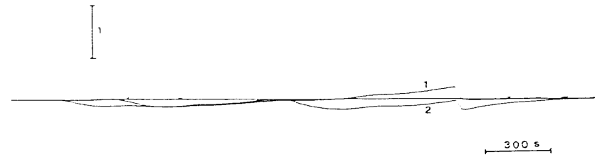
Figure 7. Process response for saw tooth disturbance and fuzzy feedforward control with (1) \alpha -composition and (2) max-min composition used for solving fuzzy relational equations
