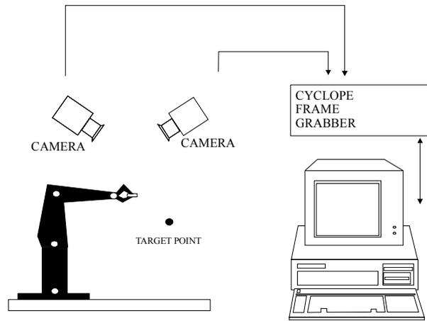
Fig.1. The system for rough target approach
