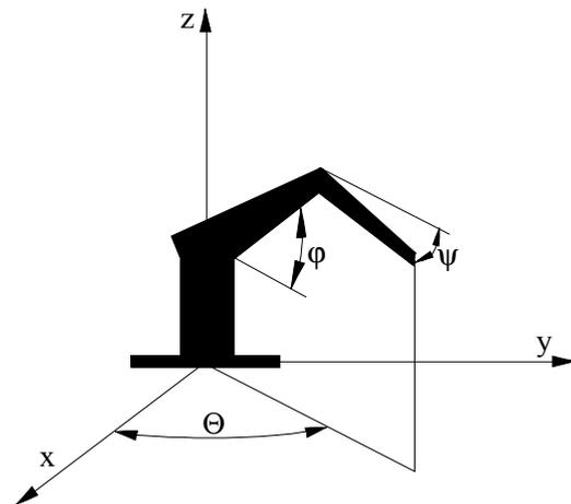
Fig.2. The robot coordinates
