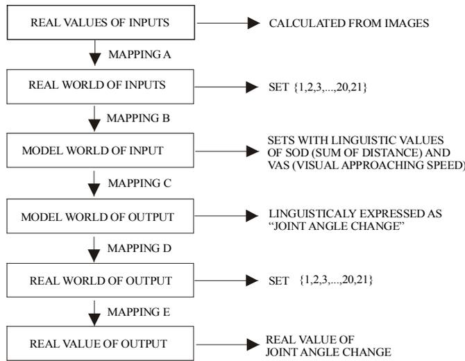
Fig.4. The whole control procedure expressed as relations between different worlds
