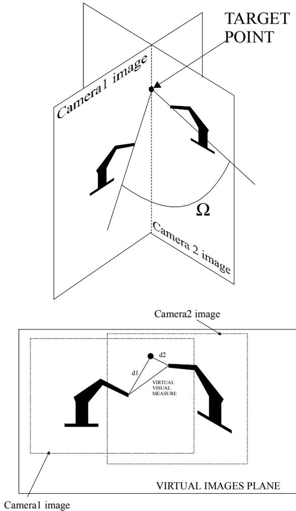
Fig.3. Construction of the virtual images plane.
